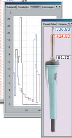
The soldering iron test shows tip temperature. The oscillations around 360°C show how the thermostat works.
